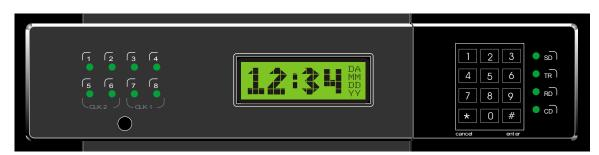
Your Master contains a lithium battery to keep the correct time when power has stopped due to an outage or the internal on/off switch. Once AC power resumes, your Master will calculate how much time your clocks lost and will automatically advance them to the correct time (this feature does not support Clock Types 14, 15 or 24).
