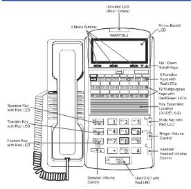
This guide is a basic suppliment to the *ADIX Quick Reference Guide* (PN 108025) and includes specific information on IX-12IPKTD IP Telephone.
