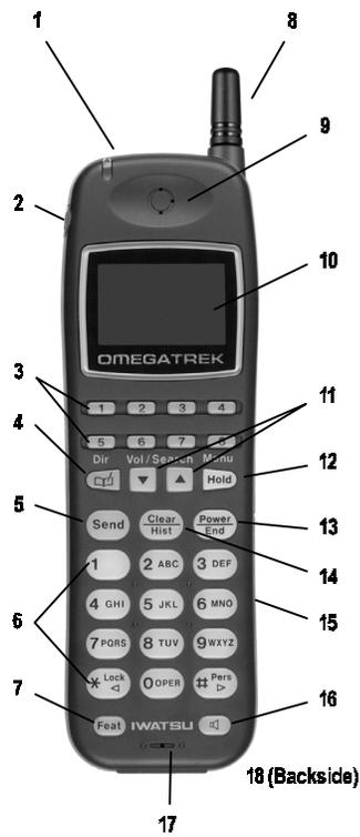
Figure 1. PS6 Digital Wireless Portable Station Features
